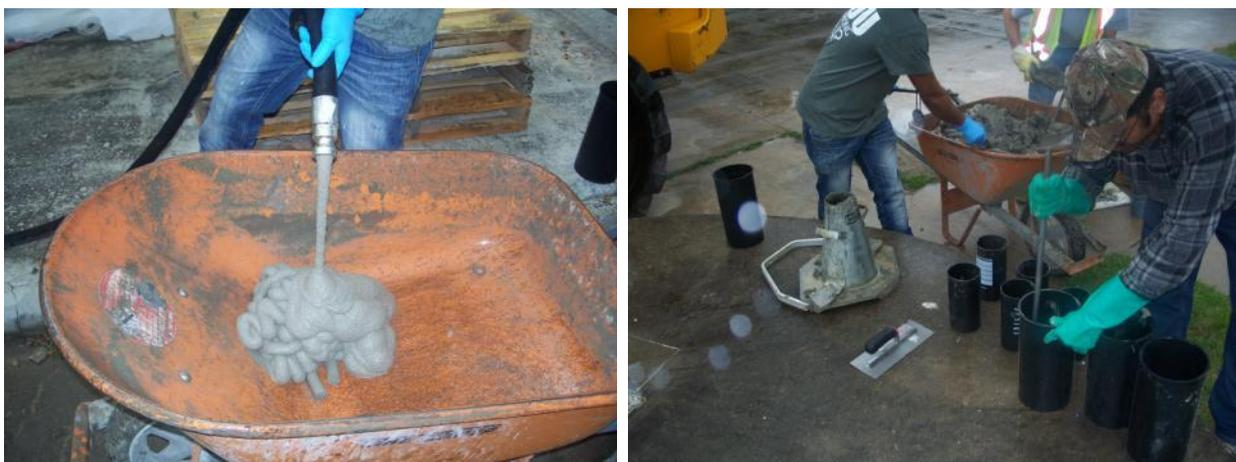
**Figure 5. Collecting Fresh Material from the Nozzle (left) and Preparing Samples (right)**
