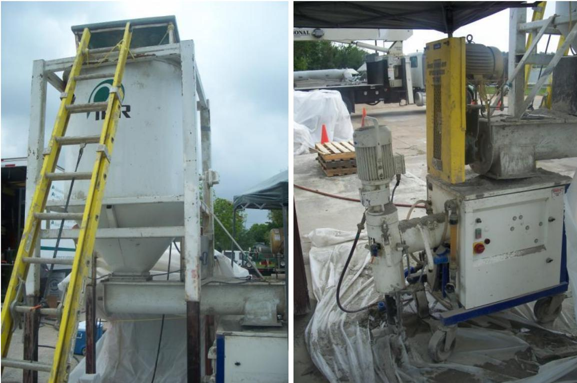
**Figure 4. Hopper (left) and Mixer (right) used for Preparing the Material**
